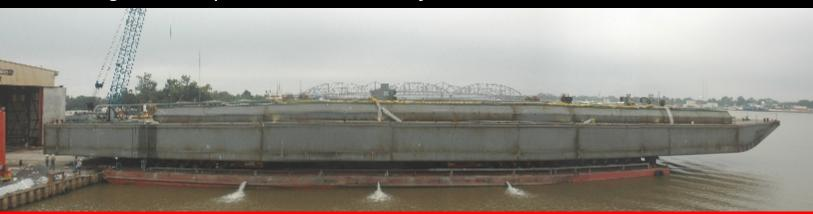
If it were three feet longer, you could play football on it. This 297' long x 54' wide barge weighing in at 950 tons was loaded out using thirty-eight axle lines of SPMT transporters onto the clients barge for launch when blast and paint are complete. Berard also moved the same size barge at the clients Orange Texas facility earlier this month. The Berard Team carried out the job in one day thanks to their hard work and dedication.
